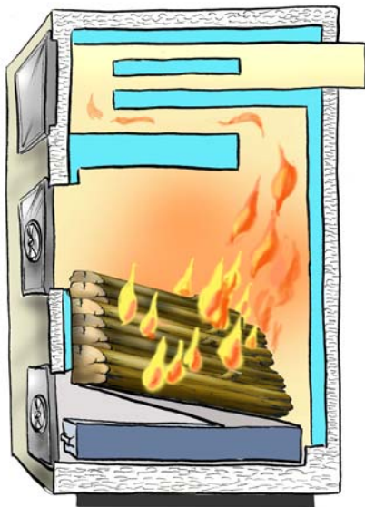
The principle of an over-fire boiler
